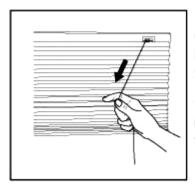
Disengage the cordlock by pulling the lift cord toward the center of the shade to raise or lower shade.
