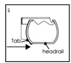
ii. Push the head rail upwards until the flexible tab at the bottom of each bracket snaps onto the back of the headrail.
